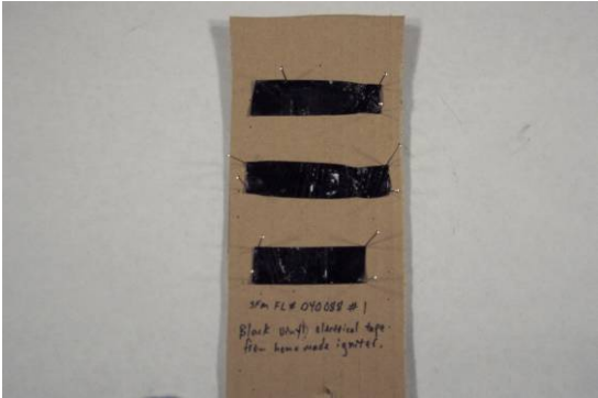
Tape can be mounted onto a piece of cardboard using pins or tape. The cardboard piece can then be taped into a box to prevent contaminating the adhesive and to prevent shifting during transport.
