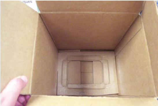
Here, the bottom is blocked in position with cardboard strips. The top is wired so as not to hit the side of the box.
