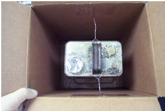
Here, the bottom is blocked in position with cardboard strips. The top is wired so as not to hit the side of the box.
